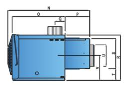
(\*) in case of long plenum (supplied only when requested) the dimensions N and P are respectively 1802mm and 1003mm
